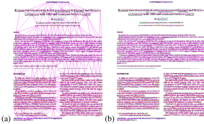
Figure 1. (a) A Voronoi word-graph. (b) The same word-graph after prune edges whose weights are less than 0.5 assigned by an edge classifier.
