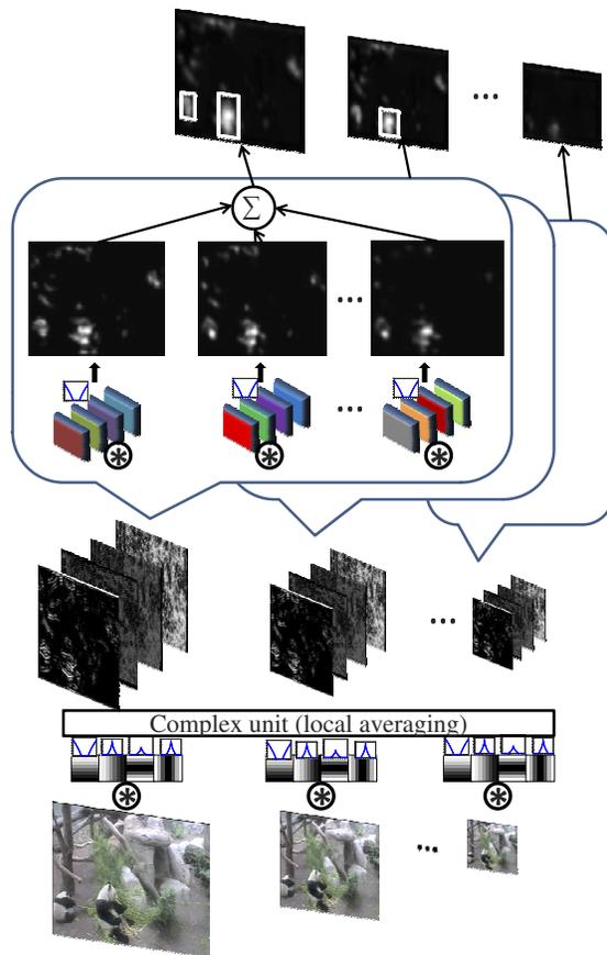
Figure 3. Architecture of the proposed template-based saliency detector. DCT features are used in the first network layer, and saliency templates in the second. The saliency computation is repeated at multiple scales.
