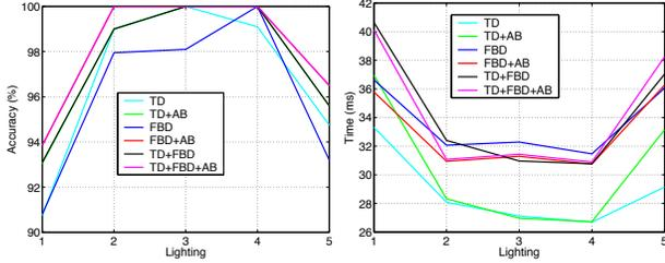
Figure 5: Tracking rate (left) and time (right) of the different detectors as a function of scene lighting condition.
