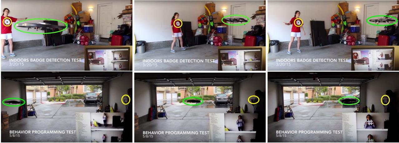
Figure 7: Experiments on the overall performance of the UAV control algorithm. Top: the UAV follows a user as she moves in 3D space. Bottom: The user successively displays two badges that command the UAV to move closer or farther away. In all images, a green (yellow) ellipse is used to indicate the position of the drone (badge). Videos of these experiments are available at [2].
