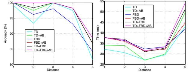
Figure 6: Tracking rate (left) and time (right) of the different detectors as a function of badge-drone distance.
