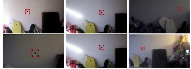
Figure 4: Badge detections over a set of images collected for different badge-drone distances and scene illuminations. Top: images collected at the same distance for different illuminations. Bottom: images collected at multiple distances.
