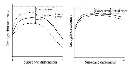
Fig. 1. Upper bound, lower bound, and actual probability of error as a function of subspace dimension. Left: dependent features. Right: independent features.
