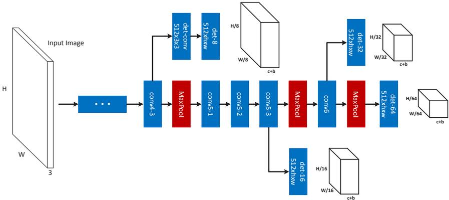
**Fig. 3.** Proposal sub-network of the MS-CNN. The bold cubes are the output tensors of the network.  $h \times w$  is the filter size,  $c$  the number of classes, and  $b$  the number of bounding box coordinates.
