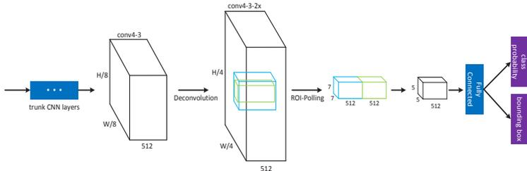
**Fig. 4.** Object detection sub-network of the MS-CNN. “trunk CNN layers” are shared with proposal sub-network.  $W$  and  $H$  are the width and height of the input image. The green (blue) cubes represent object (context) region pooling. “class probability” and “bounding box” are the outputs of the detection sub-network.
