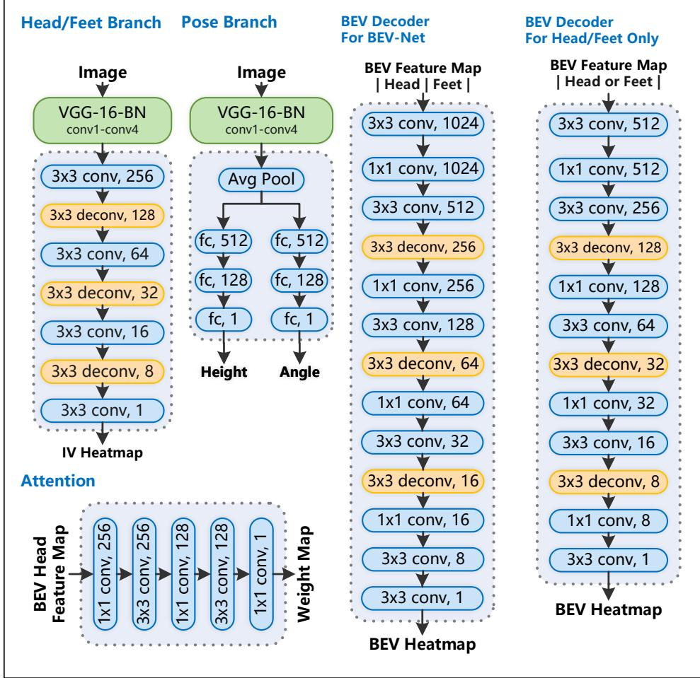
Figure 3: Network architectures. From left to right: IV (head/feet) branch, pose branch, BEV branch. The left bottom is the attention module. All conv layers have stride  $s = 1$ ; deconv layers use stride  $s = 2$ . Nonlinearity, dropout [11] and batch normalization [3] omitted between some layers for simplicity.
