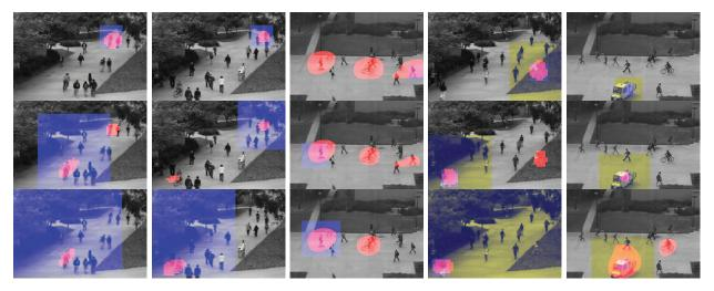
Fig. 9. Impact of context on anomaly maps. First three columns: Temporal anomalies, cell coverage at different HMDT layers shown in blue. Last two columns: Spatial anomalies, example center (surround) windows shown in blue (light yellow).
