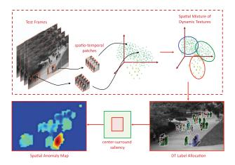
Fig. 2. Spatial anomaly detection using center-surround saliency with MDT models.
