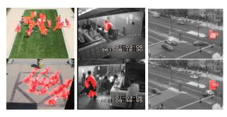
Fig. 10. Anomalies detected by H-MDT CRF on the UMN (left), Subway (center), and U-turn (right) data sets.
