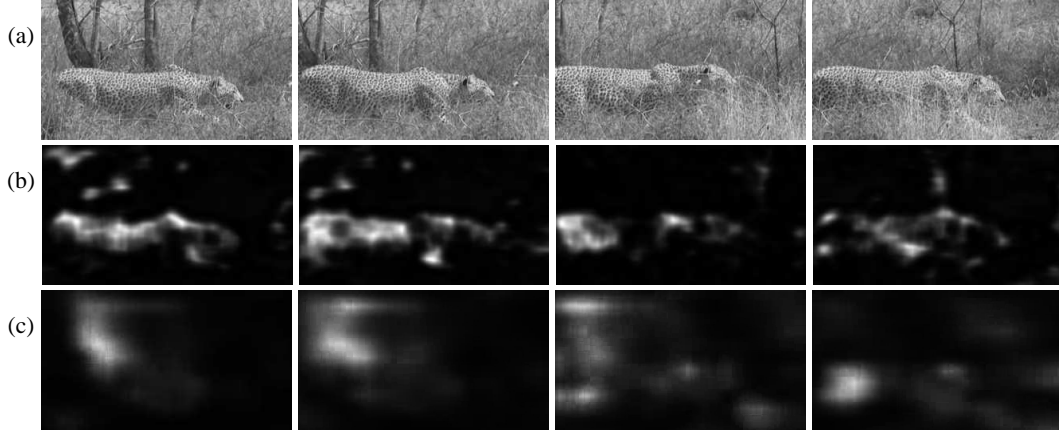
Figure 11. Saliency in the presence of ego-motion. (a) representative frames from a video sequence shot with a moving camera, (b) the saliency map produced by the motion-based discriminant saliency detector, and (c) the “surprise” maps by the model of Itti & Baldi (2005).
